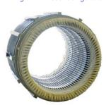
lizing packaged cores. The magnetic core consists of laminations highly compressed for mechanical strength and completely wound before the core package is inserted into the frame. This construction permits free access to the coil end-turns during manufacture and simplifies insertion of the winding and bracing systems. This visual accessibility also helps to ensure increased quality in manufacturing.
